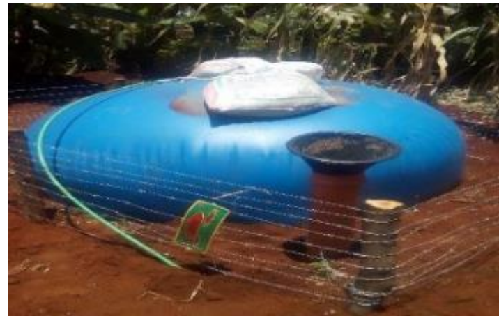
Takamoto Baloon biogas
